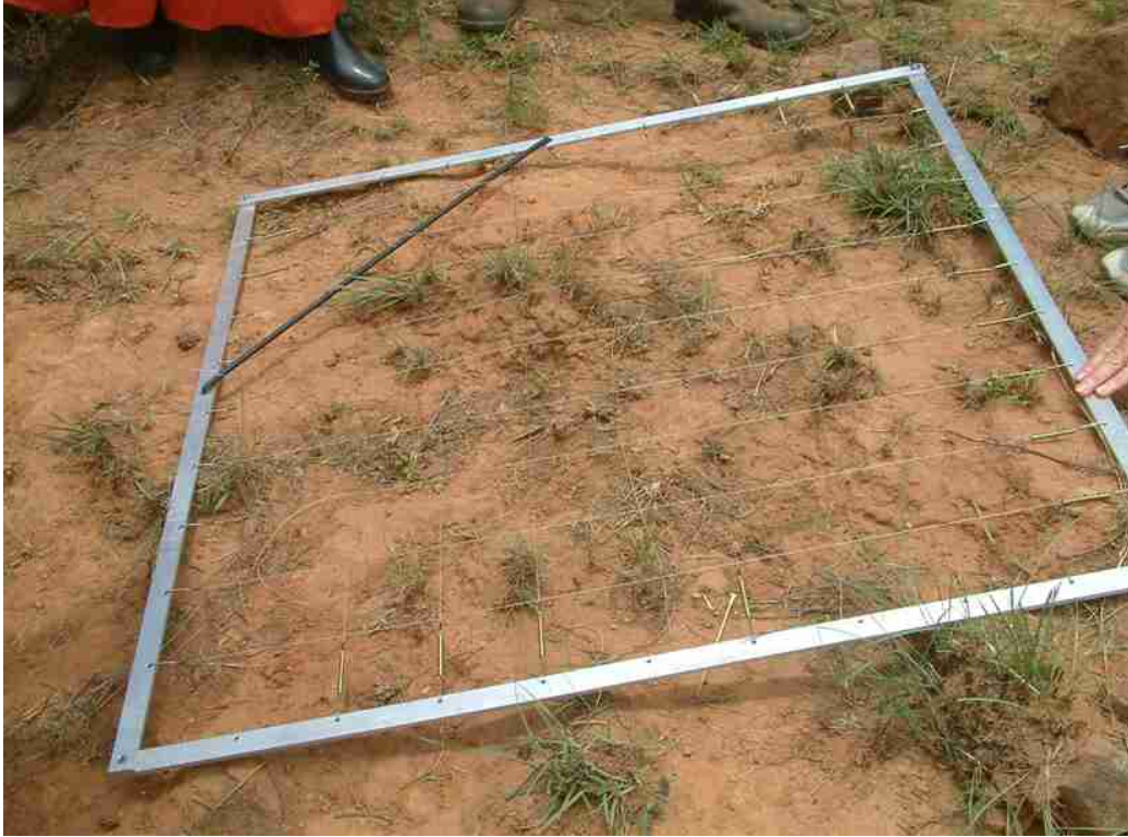
Plate 11. Quadrat used to measure basal cover of vegetation.
