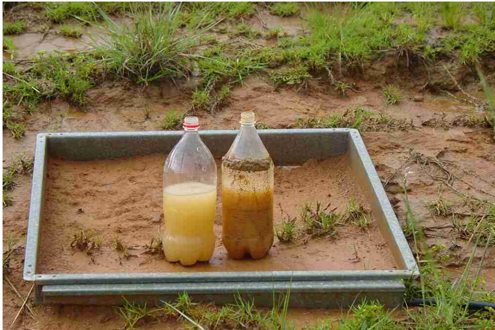
Plate 12. Runoff from plots in rehabilitated and eroded sites.
