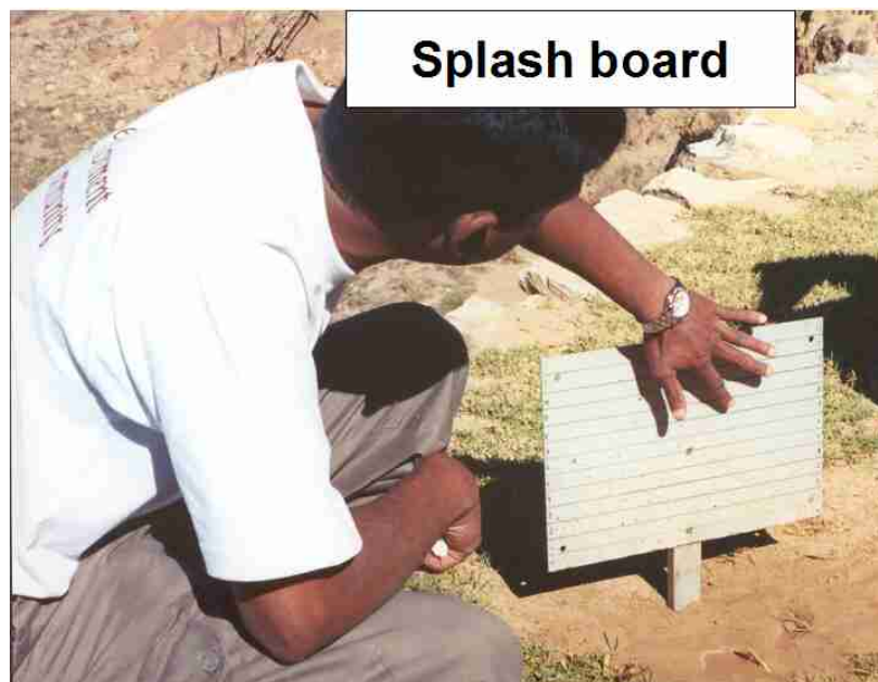
Plate 8. Splash board used to record height of rain splash.
