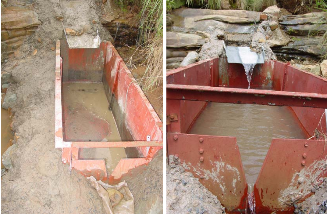
Plate 13. Portable weir in the grazed catchment. Note the flume directing the flow into the
